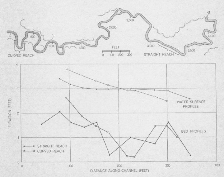
PROFILES of the water surface and bed of a small stream in Wyoming named Baldwin Creek were obtained by one of the authors (Leopold) and a colleague in 1959 during a period of maximum runoff from melting snow. Measurements were made in two places, a meandering reach and a straight reach, that were comparable in all outward aspects except sinuosity (map at top). What emerged
