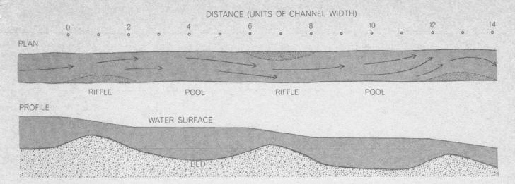
STRAIGHT REACH of a river has a more or less uneven bed that consists of alternating deeps and shallows, known to trout fishermen as riffles and pools. The humps in the stream bed that give rise to the riffles tend to be located alternately on each side of
