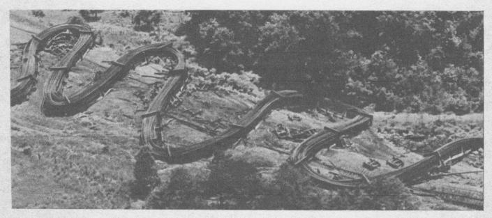
CATASTROPHIC EXAMPLE of a sine-generated curve on a much larger scale was provided by the wreck of a Southern Railway freight train near Greenville, S.C., on May 31, 1965. Thirty adjacent flatcars carried as their load 700-foot sections of track rails chained in a bundle to the car beds. The train, pulled by five locomotives, collided with a bulldozer and was derailed. The violent
