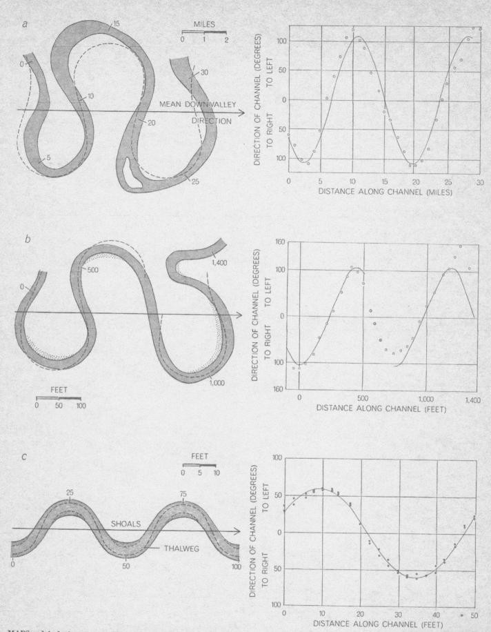
MAPS at left depict segments of two typical meandering streams, the Mississippi River near Greenville, Miss. (a), and Blackrock Creek in Wyoming (b), as well as a segment of an experimental meander formed in a homogeneous medium in the laboratory (c). Measurements of the angular direction of the channels with respect to the mean downstream direction were made at regular inter-
